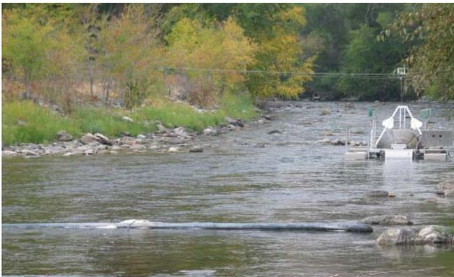
This upstream view of the Entiat River shows biologic monitoring tools. The gray pipes contain part of the PIT tags antenna system and the stainless steel “boat” with nets is the rotary screw trap.
